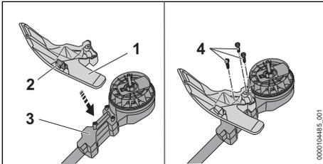
The line limiting blade (2) has already been installed in the deflector (1) and must not be removed.
